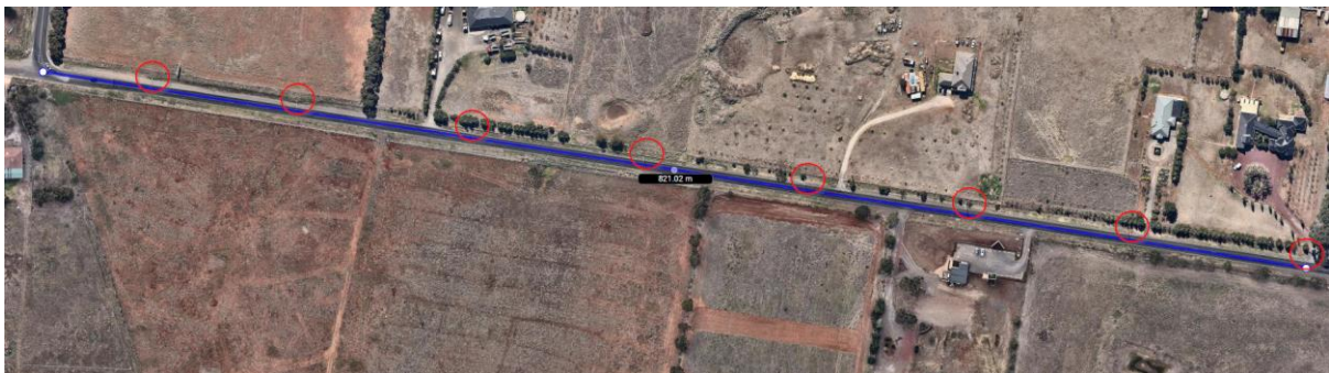
Figure 21 – Aerial imagery measurement of sight distance using telephone poles as landmarks
