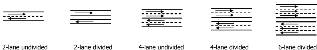
Figure 12 - Explanation of carriageway types (Source: TMR, 2017)
