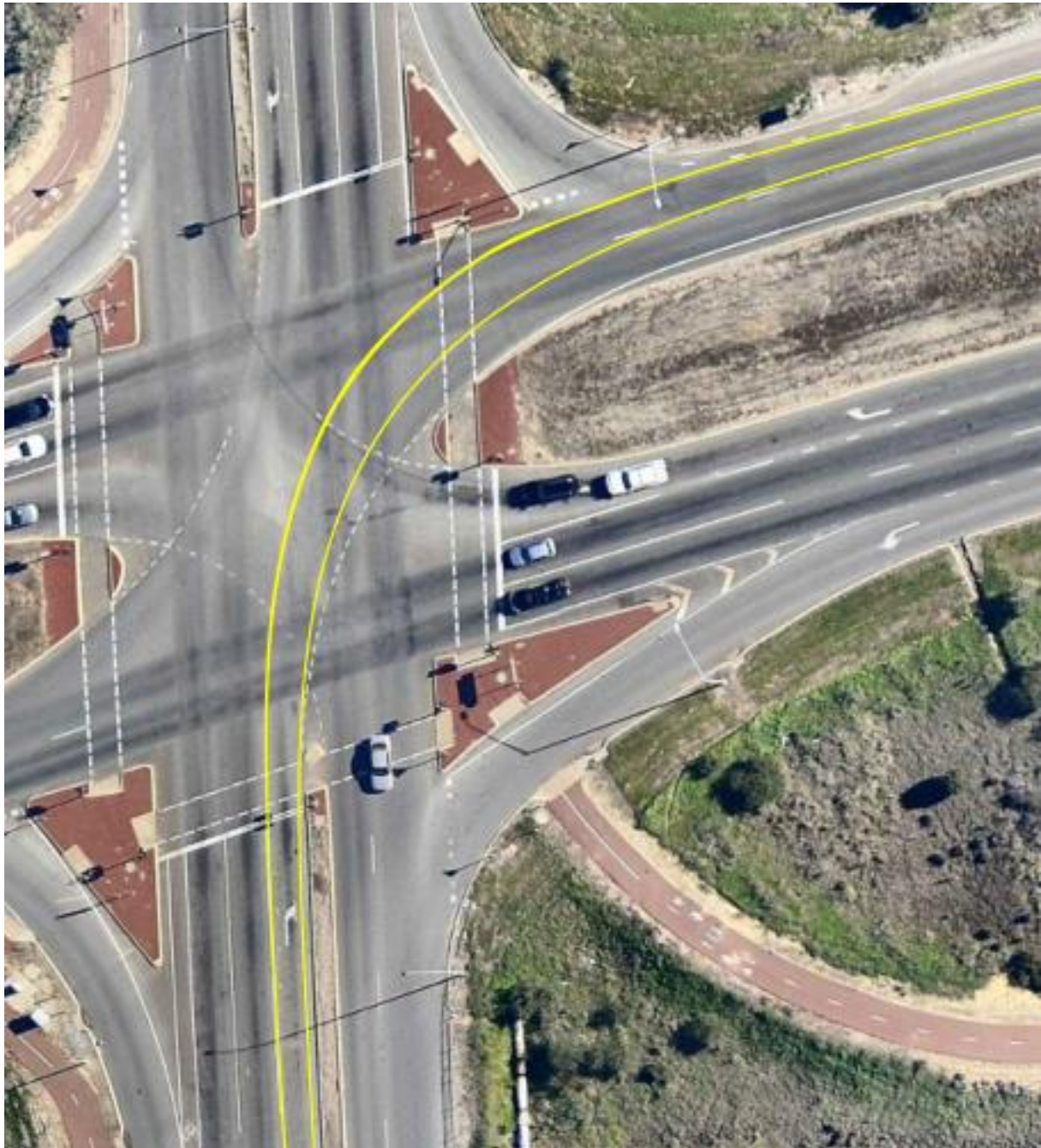
Figure 31 – A-double right turn swept path overlay
