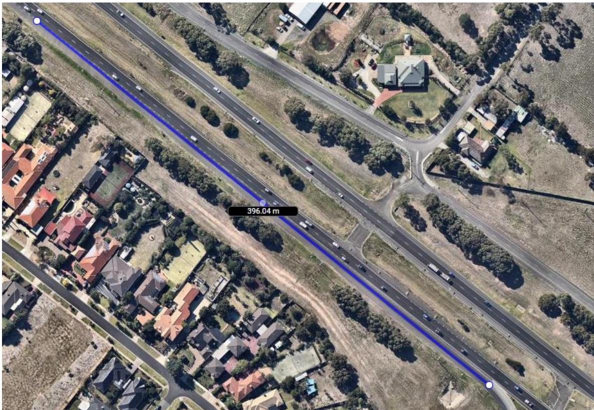
Figure 25 – Aerial imagery measurement of acceleration lane length
