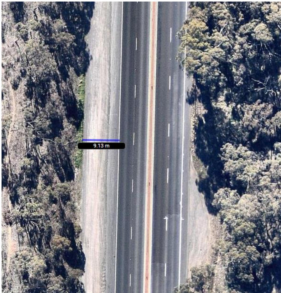
Figure 33 – Aerial imagery measurement of off-road parking clearance
