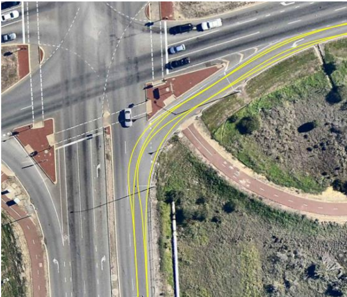
Figure 30 – A-double left turn swept path overlay
