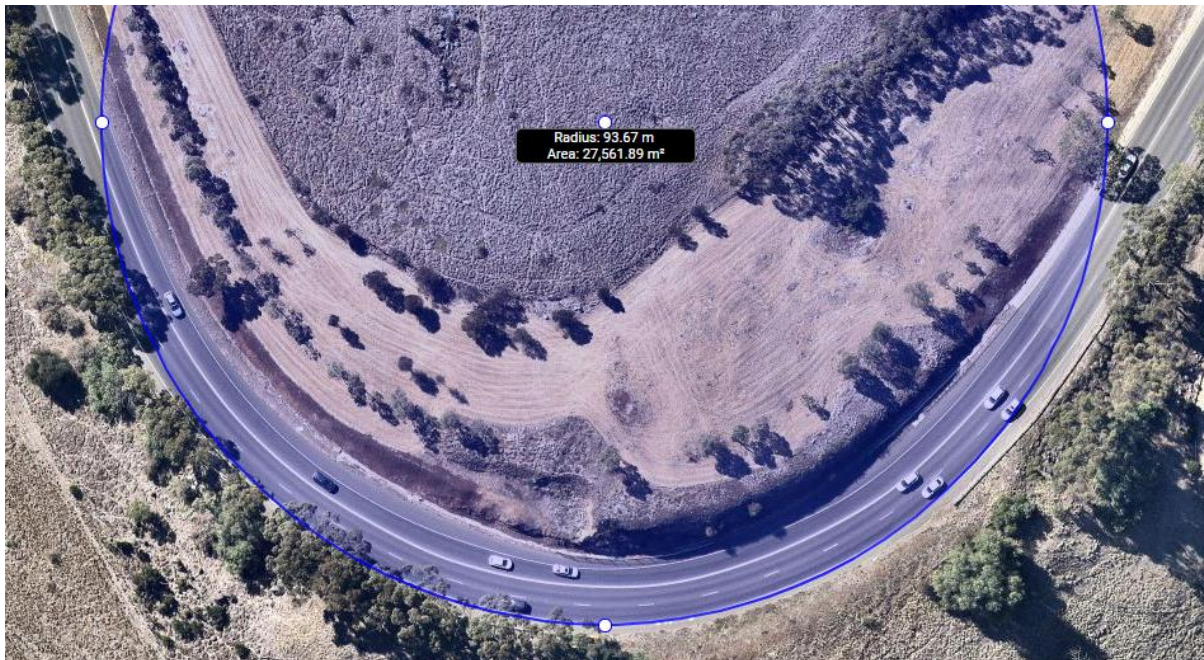
Figure 17 – Aerial imagery measurement of curve radius
