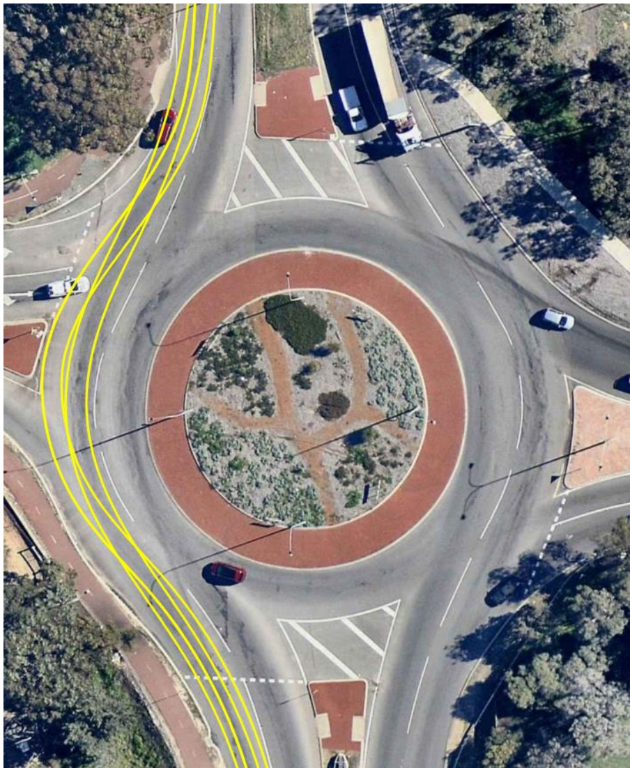
Figure 32 - A-double roundabout swept path overlay
