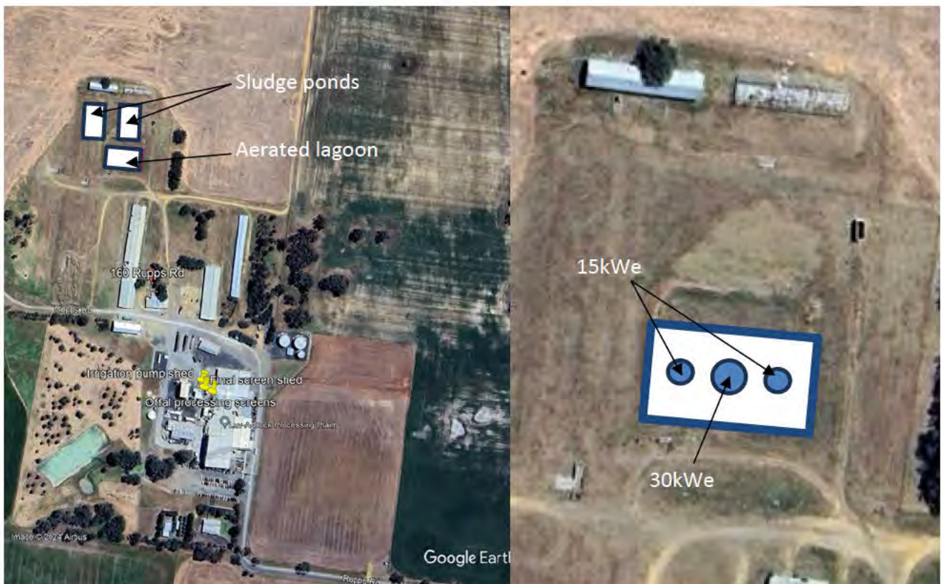
Figure 4: Preliminary layout of the aerated wastewater treatment lagoon, and sludge ponds (left), and layout of the surface aerators on the aerated lagoon (right). Note that the location and layout indicated are nominal and should be the subject of detailed site investigations to confirm a preferred location and design.
